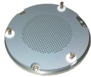
The inner grid (the Beam grid) has a voltage applied which is equal to the energy of the ion beam the user wishes to generate. The outer grid is held at earth potential. This potential difference between the grids creates a field gradient which acts to draw ions from the plasma and through the holes in the outer grid. The multiple 'beamlets' combine to form one broad ion beam which emerges into the chamber.
