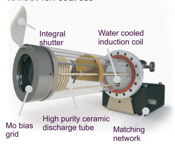
The RFMax ion sources are designed for use in UHV or HV deposition systems for applications where a broad, energetic beam of ions is required with a moderately low energy spread. The sources can generate ion beams from 50eV up to 1000eV and with beam currents between 10mA and 150mA. The beams have a typical divergence of 7 degrees when using nominally flat grids. Optionally, convex or concave grids may be mounted to give divergent or focussed beams, respectively.
